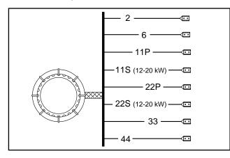
Figure 8. Stator Winding Leads
